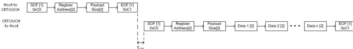
Figure 23. Register read through UART communication
